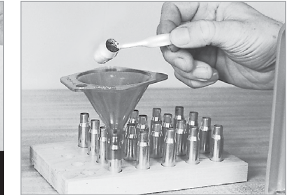
⑦ CHARGE THE CASE Regardless of how you charge the case, be absolutely certain you have the correct amount and type of powder for the bullet you have selected. NEVER try to seat the primer deeper after the powder has been added.
