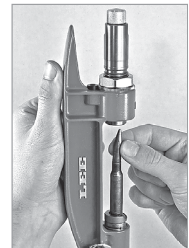
⑨ SEAT THE BULLET Place a bullet on the case mouth and guide it into the die. Raise the ram to the top and withdraw. The adjusting screw controls the bullet seating depth. Adjust to suit. Usually, seating to the same depth as a factory round works fine. If you desire to crimp, be sure the bullet crimp groove is almost completely inside the case. Then screw the die in just enough to apply a good crimp. Attempts to apply excessive
