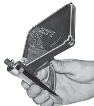
Auto Prime XR is hand held and requires special, but inexpensive shell holders.
