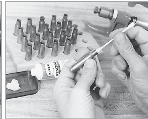
Be sure to lube the inside of the case neck with a cotton swab.
