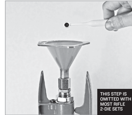
⑥ INSERT a Breech Lock bushing and screw the Expanding Die one turn short of touching the shell holder. This die flares the case mouth for easy bullet insertion. Turn deeper to increase the flare. Adjust to minimum flare needed to start the bullet. Powder may be added through Lee Expanding Die.
